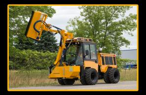
The Trackless Boom Flail Mower is perfect for those difficult, unsafe or impossible areas to mow. Ditches, steep inclines, over guard rails and waters-edge are areas in which the boom flail excels. Hydrostatic speed control allows the operator to react to oncoming obstacles for optimum safety and productivity.
