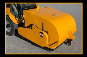
The winter battle can leave a considerable accumulation of sand and other debris on sidewalks. The Trackless Pickup Sweeper is the ideal attachment for your sidewalk spring clean up.
