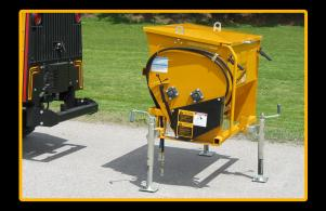
The Rear-Mount Sidewalk Spreader was specifically engineered for sidewalk applications. By dispensing a 41-inch spread width, it is designed to avoid the waste and turf damage often associated with broadcast type spreaders. The delivery roller further conserves material by spreading it evenly in a diamond pattern rather than a solid layer. Making efficient use of the spread material will allow you to go farther, prolonging the need to return for a refill saving material, labour and fuel costs.
