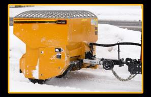
The Trackless MT tow behind spreader has a 1 yard capacity with a spread distance of up to 22 kilometers (14 miles). It is hydraulically driven and has an electric actuator which controls the spread distance. Actuator control is located in the cab next to the joystick.
