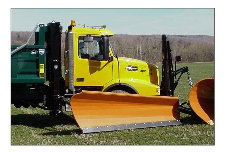
Our ACC/HCC Cable Hydraulic Wing System is modular for easy removal and installation. The ACC/HCC Wing System is designed for severe duty and offers all traditional wing functions including optional "High Rise" capabilities. A proven modern concept that offers reliability, durability and ease of operation and service.
