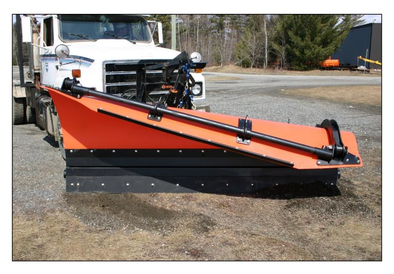
Exclusive flexible moldboard changes shape and positions for maximum versatility. Adjustable from 33" to 51" high, it also reverses in any position. Uses our ram reverse or worm gear drive frames; performance-proven features include fuel-saving polymer moldboard and trip edge design.
