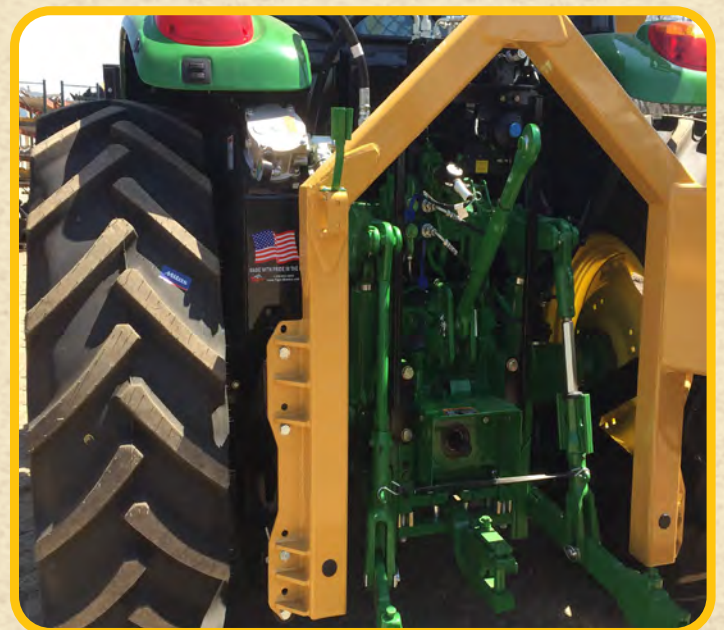
HYDRAULIC WHEEL WELL TANK
