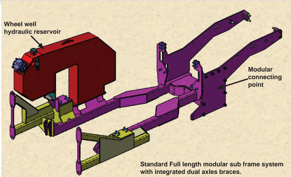
Tiger has redesigned the mounting frame for several of our tractor assemblies in a new modular format. This unique design builds additional strength into the tractor framing system while providing interchangeability. With a Tiger modular frame, changing from a boom to a side mower or from a side to a boom can be done in as little as eight hours. This increases flexibility of use without the need to buy a complete new frame and mowing system.
