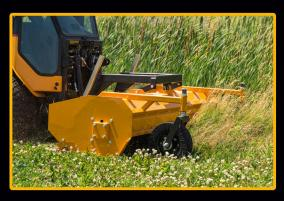
The Trackless front-mount Flail Mower was designed to cut heavier grass, weeds, scrub and light brush where a conventional rotary lawn mower could not cope. An enclosed mower housing and rubber safety skirts keep the cut grass, mulch, and other debris within the cutting chamber and enable safe mowing near roads, parks, and other busy or populated areas.
