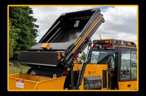
The Dump Body is an option for municipalities that wish to double the spread distance with the Rear Sidewalk Spreader before having to return for a refill. The operator spreads material until empty and then refills the rear spreader by hydraulically raising the dump body. The built-in tailgate opens and closes automatically as the dump body is raised and lowered. When the winter season is over, the dump body and its supporting frame can be unbolted and stored until the following winter.
