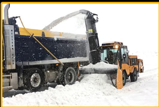
The Ribbon Snowblower is the next generation of gearbox snowblower technology from Trackless Vehicles Ltd. Designed for higher output, this snowblower outperforms all others in heavy wet snow and is extremely aggressive when cutting into frozen banks.
