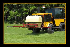
A dust control Spraying System is recommended for use with sweepers. It consists of a rear-mounted 80 U.S. gallon tank with 12 V pump, relief valve, and hoses. All MTs have electric wiring, hose and switch installed, ready for this system. A front spray bar kit must be ordered separately for each type of sweeper. A variety of different spray bars are also available for spraying salt brine, magnesium chloride, calcium chloride, etc.
