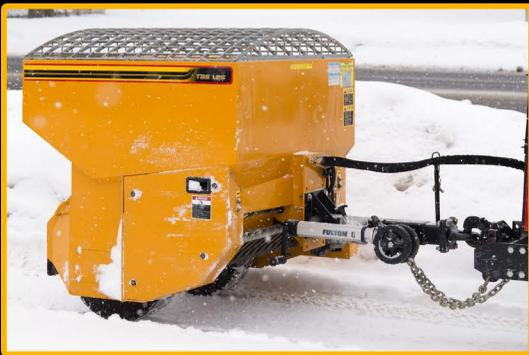
The Trackless MT tow behind spreader has a 1 yard capacity with a spread distance of up to 22 kilometers (14 miles). It is hydraulically driven and has an electric actuator which controls the spread distance. Actuator control is located in the cab next to the joystick.
