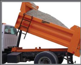
Available with either a front mount telescopic hoist or underbody hoist.
