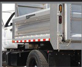
Formed sides minimize corrosion and increase overall strength.
