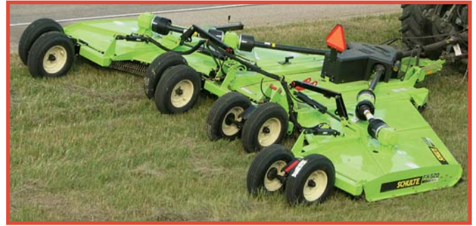
Tandem Walking Axles work great for Highway & Road-side mowing
