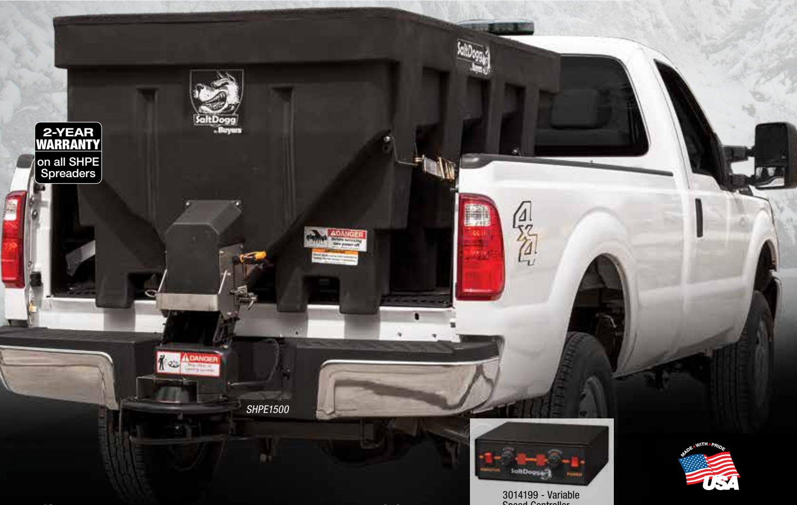
NEW high flow chute with larger 14" spinner, open trough, and shield that better protects truck from flying salt
