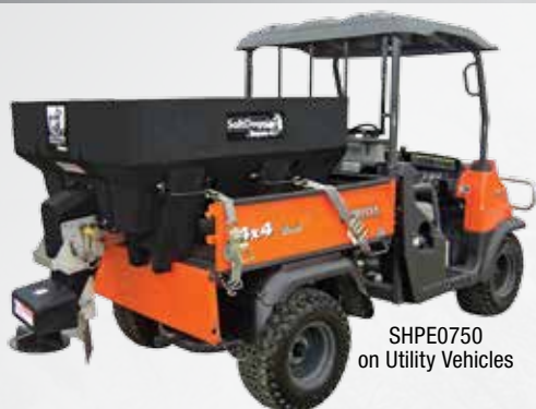
NEW high flow chute with larger 14" spinner, open trough, and shield that better protects truck from flying salt
