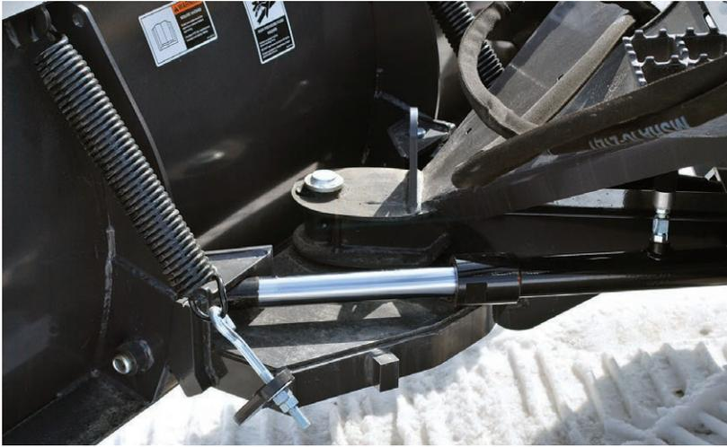
The **115 Series** angles 35° in either direction hydraulically. Equipped with a 7-gauge steel blade. Optional flap reduces snow spillage. For Large SSL, Compact Utility Loaders, Small Wheel Loaders and Backhoe Loaders.
