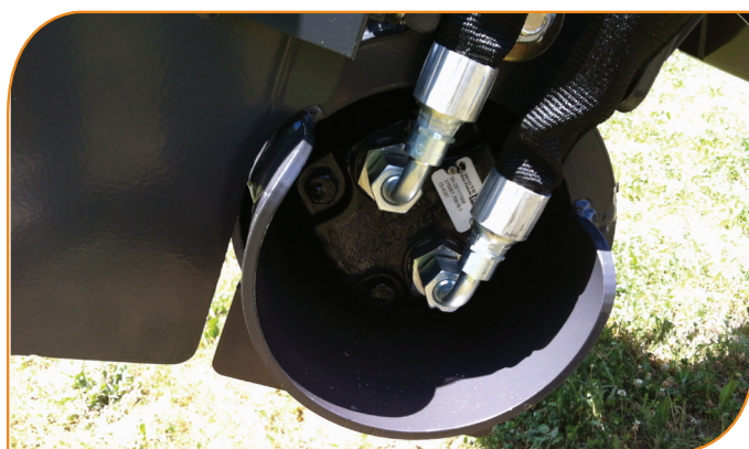
New direct drive motor protected within frame and drum.
