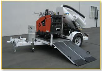
Special propane powered PV-66 Saw Trailer
