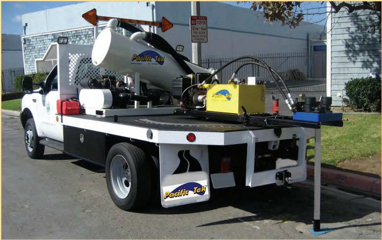
Model PT-25 Swivel Mounted Heavy Duty Valve Operator
