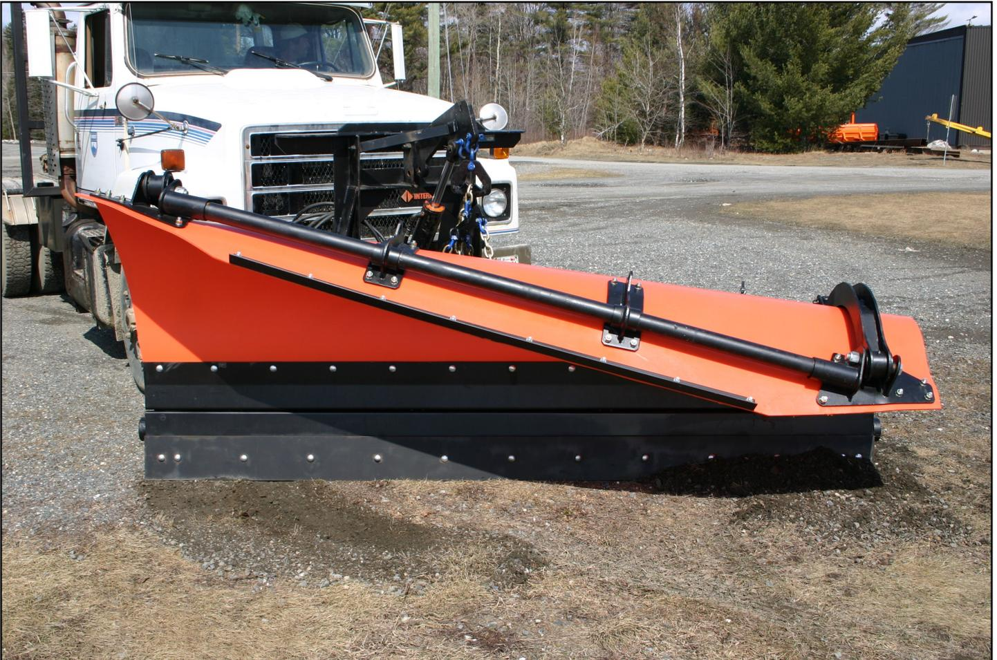
Exclusive flexible moldboard changes shape and positions for maximum versatility. Adjustable from 33” to 51” high, it also reverses in any position. Uses our ram reverse or worm gear drive frames; performance-proven features include fuel-saving polymer moldboard and trip edge design.
