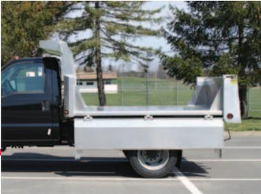
Fold down sides feature a centrally located quick release lever that extends and retracts 3/4" pins at each end using a solid linkage member. Weight-saving aluminum fold down sides are optional on steel bodies.
