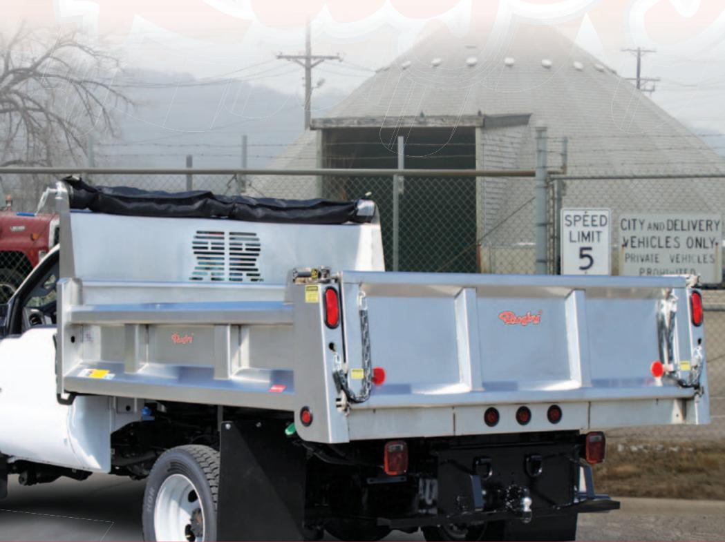
Stainless steel dump bodies from Rugby are corrosion resistant and more durable than high tensile steel.
