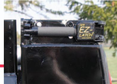
Rugby's patented and industry leading EZ-LATCH™ (located on each side of body) allows for easy body access. The latch system is designed for quick opening and slam lock operation with a cam action to draw-in upper tailgate pins.
