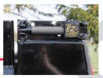
Rugby's patented and industry leading EZ-LATCH™ (located on each side of body) allows for easy body access. The latch system is designed for quick opening and slam lock operation with a cam action to draw-in upper tailgate pins.
