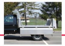
Fold down sides feature a centrally located quick release lever that extends and retracts <sup>3</sup>/<sub>4</sub>" pins at each end using a solid linkage member. Weight-saving aluminum fold down sides are optional on steel bodies.
