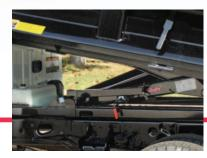
Low Mount Hoist The Eliminator LP's lower mounting height improves the body's overall stability. Actual mounting height 7 5%".
