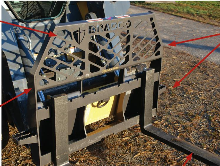
Angled side corners and step for easy and safe side access in and out of operator
