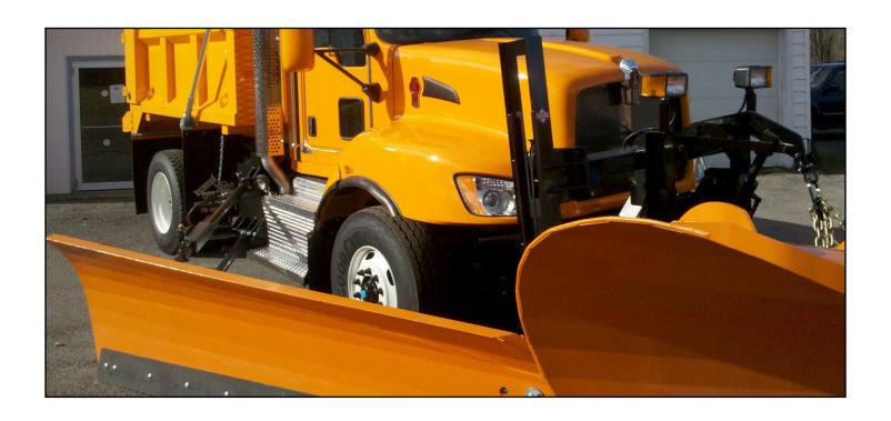
The P89/FP88 patrol wing system by American Sno-plows is designed for heavy duty snow and ice control with limited benching capabilities. Durable frame design with minimum chassis footprint for compact installation.
