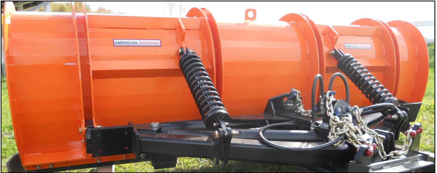
The CSA reversible plow offers a full moldboard trip configuration with adjustable compression spring arm trip assembly for positive tripping action in heavy duty snow removal situations. Designed with a j-curve moldboard with integral snow shield to minimize blow back over the plow and maximize productivity. Hydraulically reversible to meet all your snow removal requirements.
