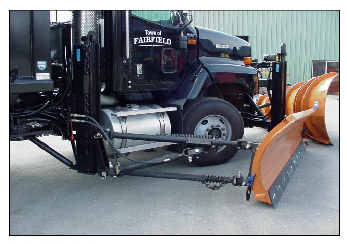
Our ACP Full Hydraulic Wing System features a modular concept for easy removal and installation. Side wing lift and shelving is accomplished by hydraulic cylinders with no cable attachments. Choice of low rise or high rise lift front and rear towers are available. Severe service wing braces and independently operated wing arm cylinder. Highway high speed leveling capabilities as well as widening operations.
