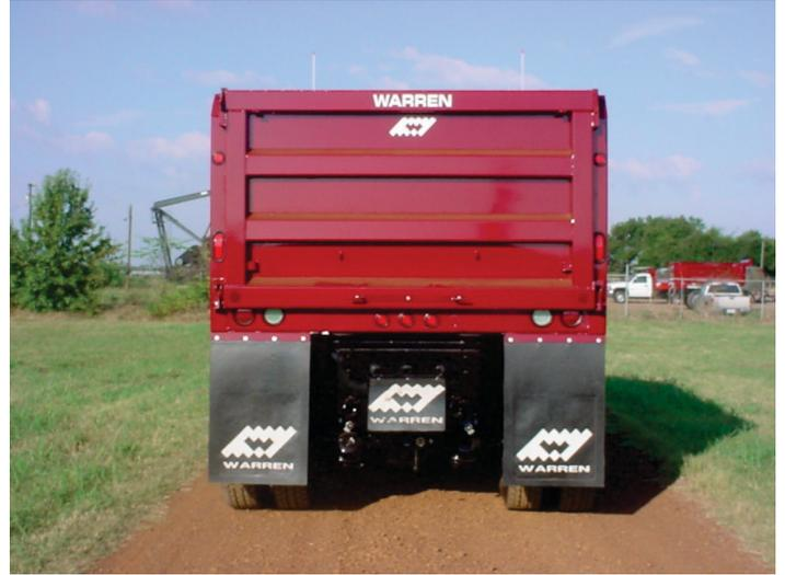
Ws700 Shown with optional metal boards, tarp system, lights in rear crossmember, and tow package.
