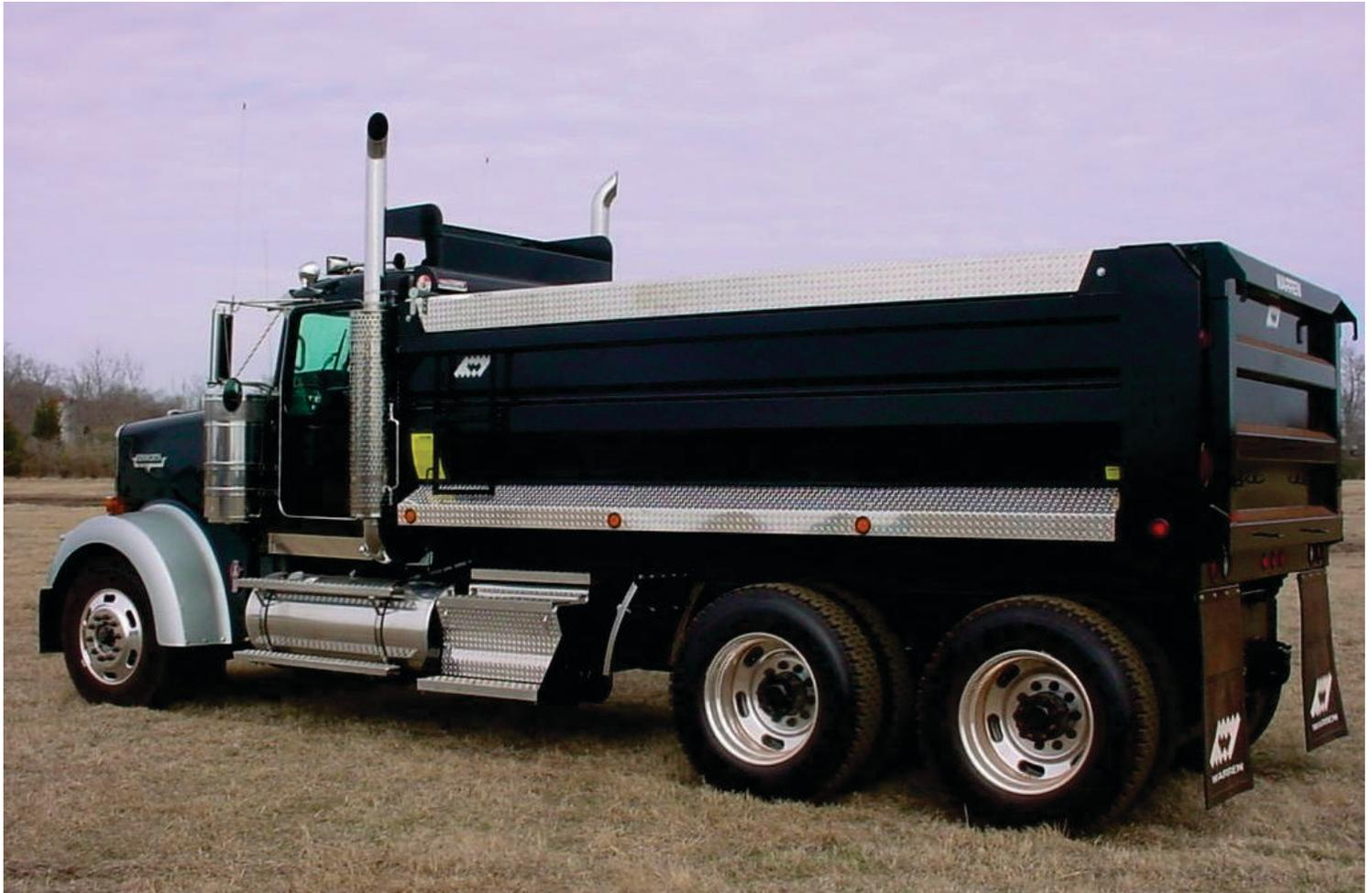
**WS700** Shown with optional metal boards w/ aluminum covers, aluminum fender covers w/ extra lighting, tow package, & pull tarp.
