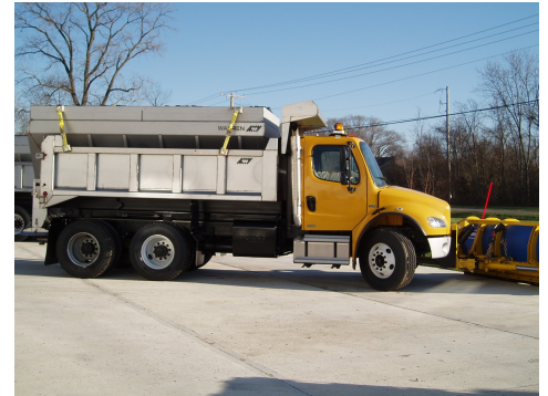
14' WXL body & E/AC2420 Spreader in 304 Stainless Steel
