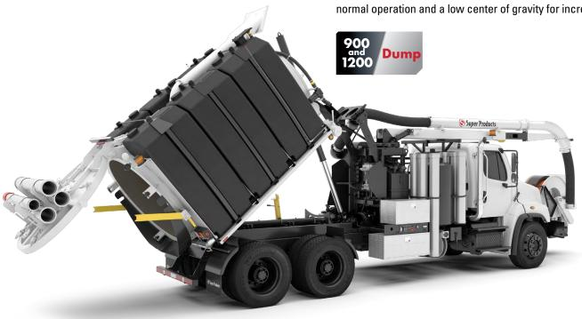
**Ejection Unloading:** The ejection unloading system is the industry's safest and most efficient removal of debris. The body raises to an 8.5° angle and the ejector plate quickly pushes out debris. This allows operators to have **the only controlled way to dump into a 48-inch container** without the need of additional containment products.
